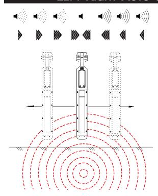
In this mode the unit will display directional arrows to the conductor. The audio indicator will provide a solid tone on one side of the conductor and a pulsed tone on the opposite side of the conductor. When the unit is centered in the electromagnetic field the tone will null and the depth will briefly display at the top of the LCD. This mode is gain independent.
