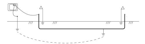
With transmitter off connect red lead to the faulted conductor and black lead to independent ground rod placed behind and in line with the conductor path.
