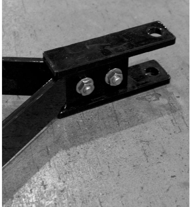
Tongue Assembled to Hitch Clevis
