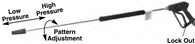
Figure 17 – Wash Wand Nozzle Adjustments
