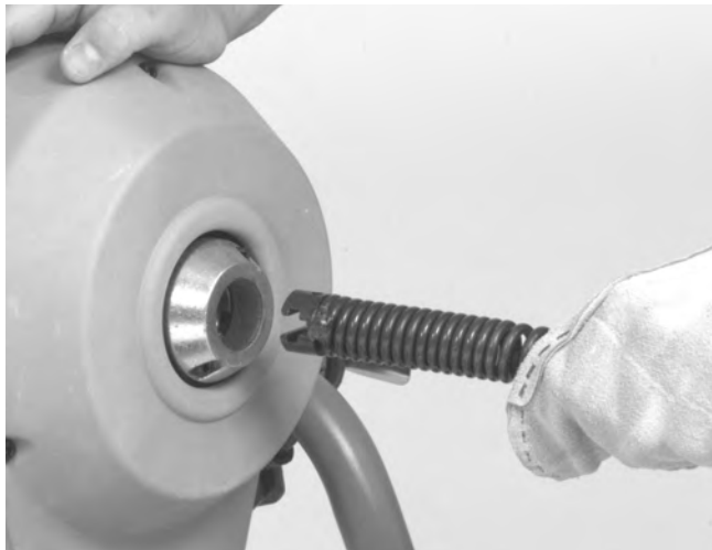
Figure 4 – Inserting Cable Into Front Of Machine
