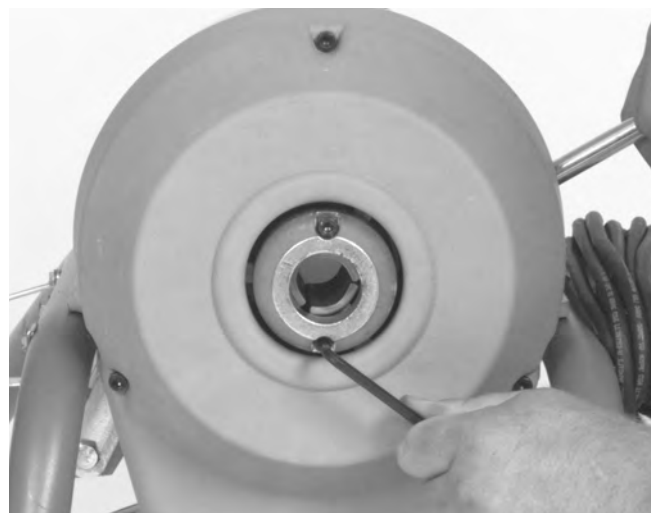
Figure 12 – Replacing Clutch Jaws
