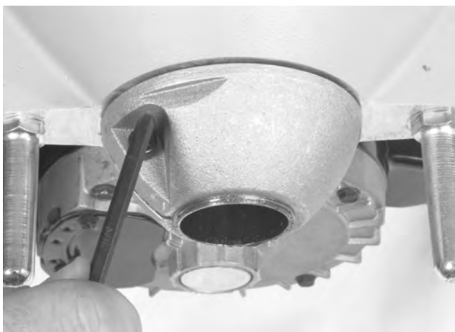
Figure 14 – Removing Clutch End Play
