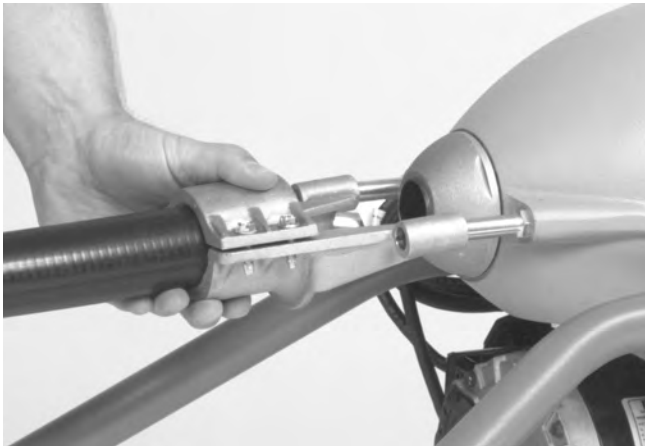
Figure 3 – Rear Guide Hose Attachment
