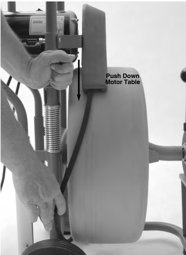
Figure 17 – Releasing Belt Tension
