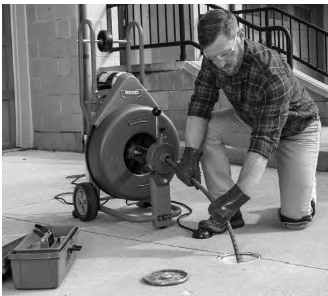
Figure 12 – In Operating Position, Manually Feeding Cable
