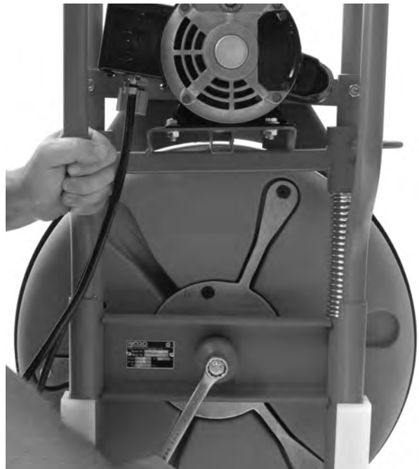
Figure 18 – Removing Drum Bolt
