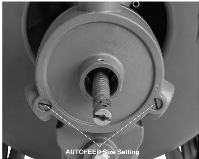
Figure 9 – AUTOFEED Size Setting
