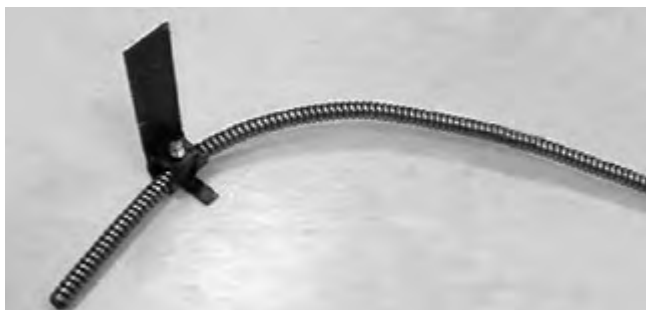
Figure 18 – Torque Arm Attached to Cable. Cable Should Be Permanently Bent as Shown with Clamp Installed Approx. 2" From End of Cable
