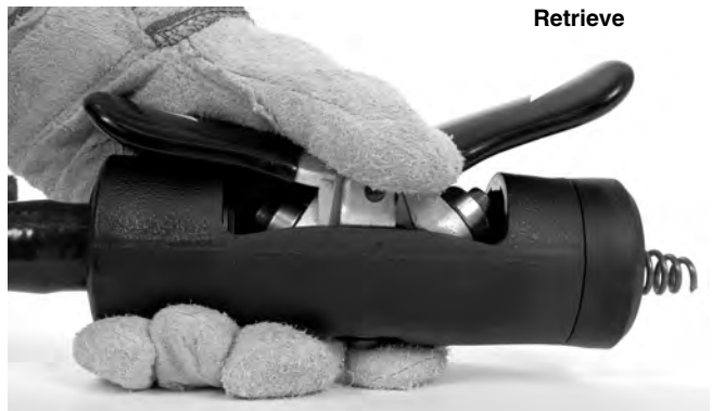
Figure 13 – AUTOFEED in Advance and Retrieve Position
