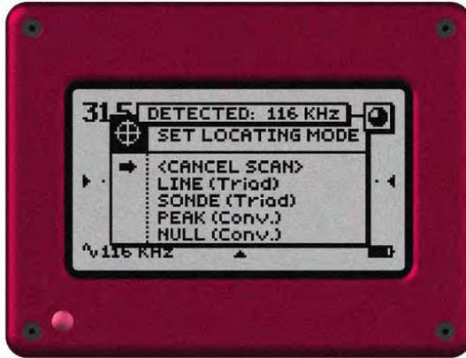
After a successful scan, the display will report as shown to the left. Having detected a signal from an active transmitter, the receiver will automatically present the "SET LOCATING MODE" menu. To continue, follow the instructions for setting the locating mode given on the following page of this manual. If you are unable to SCAN successfully, please refer to Appendix C, "Troubleshooting", for more help.
