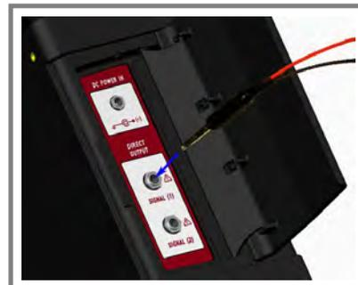
(c) Connect the black lead to a metallic stake that has been securely plunged into the ground. The amount of current generated on the target line depends largely on the nature of this ground connection. For longer traces, place the ground stake as far away from the red clip as possible. If little signal is required for the tracing job, then the user can even leave the black lead unattached and laying on the ground some distance from the red lead. This is referred to as an "off-ground" condition.
