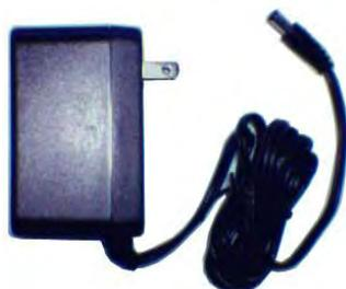
[6] **External AC Power Supply.** This two-prong AC wall socket adapter that supplies unlimited power to the 23X Transmitter. This is especially useful when the 23X drives heavy loads at audio frequencies for long duration. [Specs: Input = 120 VAC, 60 Hz, 22 W; Output = 15 VDC @ 1 Amp; Plug dimension =  $\varnothing$ 2.5 x 5.5 mm]
