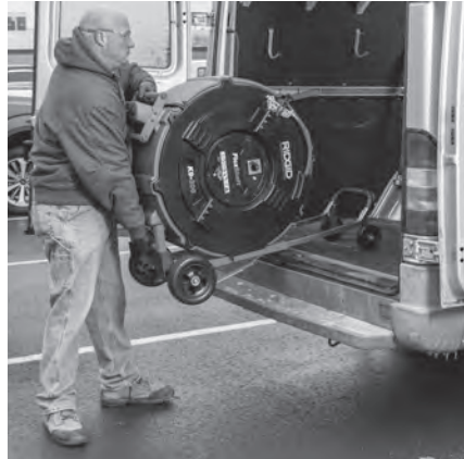
Figure 17 – Lifting Unit Onto Vehicle
